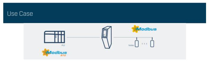
The Anybus Communicator Modbus RTU Server to Modbus TCP Client enables you to connect any Modbus RTU control system to any Modbus TCP control system.
