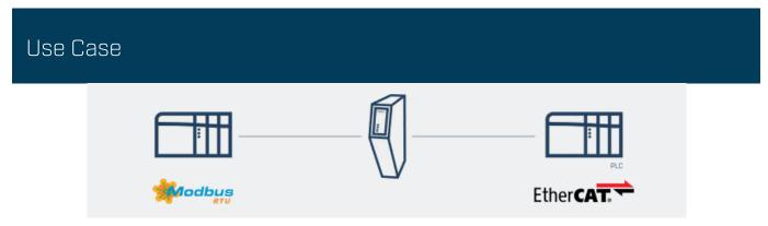
The Anybus Communicator Modbus RTU Server to EtherCAT Subdevice enables you to connect any Modbus RTU control system to any EtherCAT control system.
