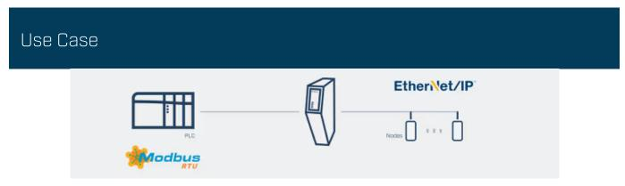
The Anybus Communicator EtherNet/IP scanner to Modbus RTU server enables you to connect any EtherNet/IP device to Modbus RTU control systems.
