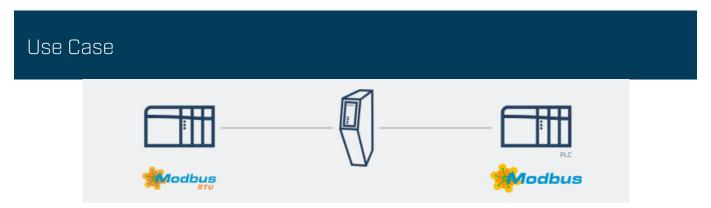
The Anybus Communicator Modbus RTU Server to Modbus TCP Server enables you to connect any Modbus RTU control system to any Modbus TCP control system.
