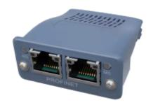
Enable communication between industrial devices and PROFINET-IRT networks
