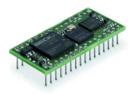
An embedded SoC web controller with a DIL32 footprint for the industrial control and communications market.
