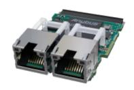
Enable communication between industrial devices and CC-Link IE TSN networks
