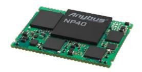
Enable communication between industrial devices and Modbus TCP networks
