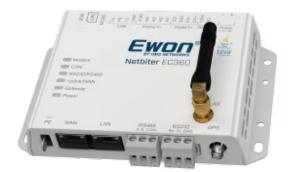
Remote communication gateway exchanging data over Cellular 4G or Ethernet to the Netbiter Argos IIoT platform
