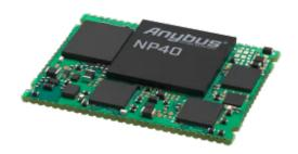
Enable communication between industrial devices and EtherNet/IP networks
