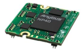
Enable communication between industrial devices and Ethernet/IP networks
