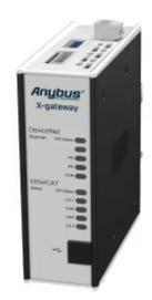
A protocol converter that connects DeviceNet devices to EtherCAT PLCs
