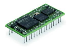
An embedded SoC web controller with a DIL32 footprint for for IEC 61131-3 runtime system
