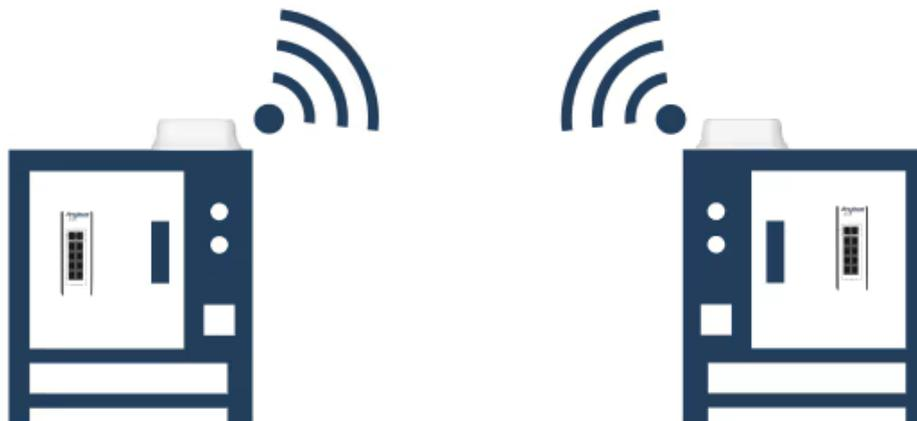
The Anybus Wireless Bolt II is configured as an access point and mounted on a cabinet to allow wireless access between an HMI and the equipment in the cabinet. The Bolt II is powered by a PoE switch inside the cabinet.
