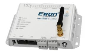
Remote communication gateway exchanging data over Cellular 4G or Ethernet to the Netbiter Argos IIoT platform
