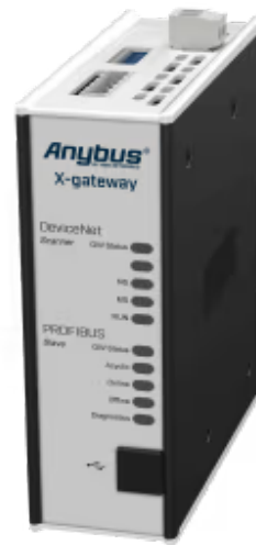
A protocol converter that connects DeviceNet devices to PROFIBUS PLCs
