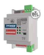
Hitachi to BACnet/IP & MS/TP - 1 indoor unit
