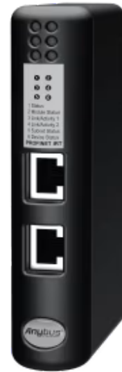
A protocol converter that connects CANopen devices to PROFINET-IRT PLCs
