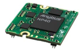
Enable communication between industrial devices and EtherCAT networks
