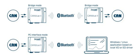
Ixxat CANblue II is operated in bridge mode as a device pair that connects two remote CAN systems via Bluetooth. This allows e.g. the connection of moving components, the avoidance of slip ring connections or the connection of devices for which wiring is no option. When using the PC operating mode, a CANblue II is connected via the PC's internal Bluetooth interface. This enables easy, wireless access to CAN systems, e.g. for maintenance, configuration or analysis.
