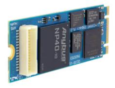
Connects computers and embedded systems to PROFINET IRT networks
