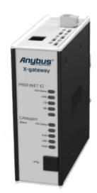
A protocol converter that connects CANopen and PROFINET-IO control systems
