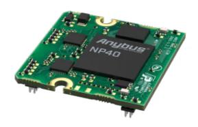
Enable communication between industrial devices and Modbus-TCP networks
