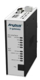
A protocol converter that connects AS-Interface to OPC UA-MQTT information systems
