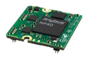
Enable communication between industrial devices and DeviceNet networks
