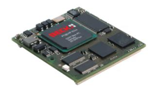
An Computer on Module built on the highly integrated 32-bit Power Architecture  $^{\text{\tiny M}}$  technology. Designed for demanding control and intensive network communication tasks.
