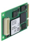
Connects computers and embedded systems to PROFINET Fiber Optic networks
