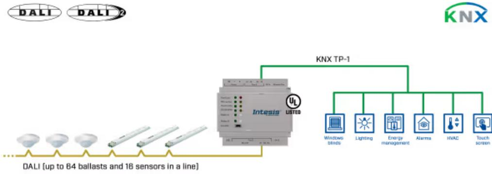
Integration of DALI drivers and sensors into a KNX installation.
