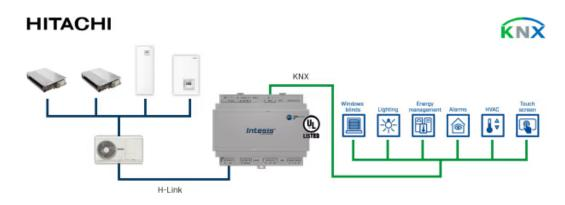
Integration example: when using the gateway to integrate mixed unit types like VRF and Ait-to-water systems.
