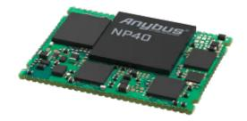
Enable communication between industrial devices and PROFINET networks
