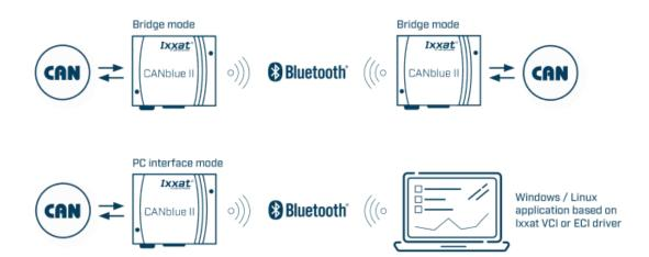
Ixxat CANblue II is operated in bridge mode as a device pair that connects two remote CAN systems via Bluetooth. This allows e.g. the connection of moving components, the avoidance of slip ring connections or the connection of devices for which wiring is no option. When using the PC operating mode, a CANblue II is connected via the PC's internal Bluetooth interface. This enables easy, wireless access to CAN systems, e.g. for maintenance, configuration or analysis.
