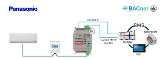
\*BACnet IP or BACnet MSTP communication selectable from switch configuration.
