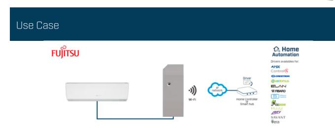
Integration of Fujitsu Domestic and VRF Air Conditioners Units into a Home Automation installation.
