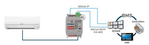
\*BACnet IP or BACnet MSTP communication selectable from switch configuration.
