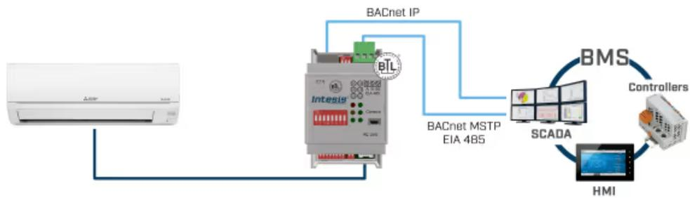
*\*BACnet IP or BACnet MSTP communication selectable from switch configuration.*
