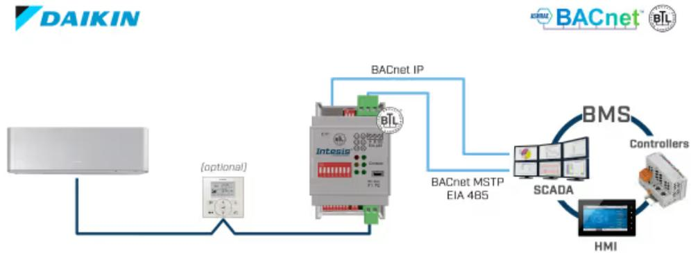
*\*BACnet IP or BACnet MSTP communication selectable from switch configuration*
