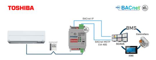
\*BACnet IP or BACnet MSTP communication selectable from switch configuration
