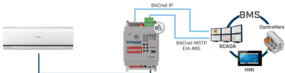
*\*BACnet IP or BACnet MSTP communication selectable from switch configuration.*
