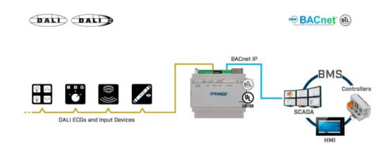
Integration of DALI drivers and sensors into a BACnet installation.
