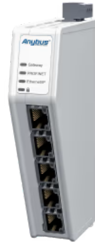
A protocol converter that connects PROFINET IO and EtherNet/IP control systems
