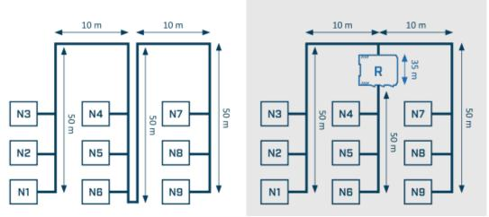
CAN repeaters can be used to better adapt the cable routing to the ambient conditions. Stub lines can be made and the bus structure can be expanded to a star/tree structure, which saves cable lengths. Shorter cable lengths reduce interference on the signal lines and enable higher bit rates. Segments connected via repeaters are galvanically decoupled and therefore offer overvoltage protection for connected participants.
