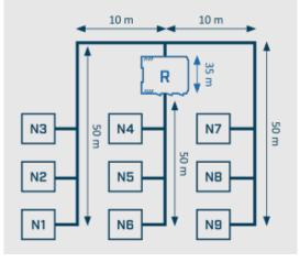
CAN repeaters can be used to better adapt the cable routing to the ambient conditions. Stub lines can be made and the bus structure can be expanded to a star/tree structure, which saves cable lengths. Shorter cable lengths reduce interference on the signal lines and enable higher bit rates. Segments connected via repeaters are galvanically decoupled and therefore offer overvoltage protection for connected participants.
