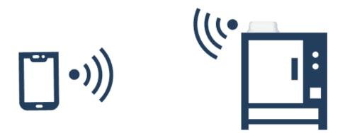
A wireless network is extended between two cells by mounting a pair of Anybus Wireless Bolt II set to cable replacement mode on top of the industrial control cabinets. The Bolt II is powered by a PoE switch inside the cabinet.
