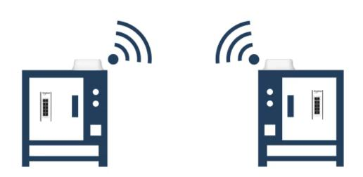
The Anybus Wireless Bolt II is configured as an access point and mounted on a cabinet to allow wireless access between an HMI and the equipment in the cabinet. The Bolt II is powered by a PoE switch inside the cabinet.
