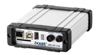
Configurable automotive platform (1 x FlexRay, 6 x CAN + 2  $\times$  CAN FD)
