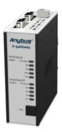
A protocol converter that connects PROFIBUS devices to EtherNet/IP PLCs
