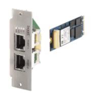
Connects computers and embedded systems to PROFINET IRT networks
