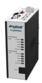
A protocol converter that connects PROFIBUS and PROFIBUS control systems
