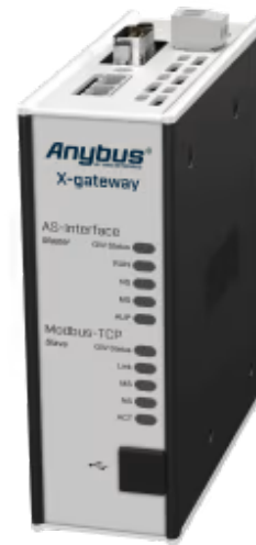
A protocol converter that connects AS-Interface devices to Modbus TCP PLCs
