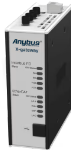
A protocol converter that connects EtherCAT and Interbus FO control systems
