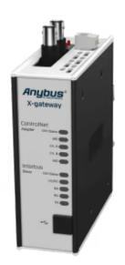
A protocol converter that connects ControlNet and Interbus CU control systems
